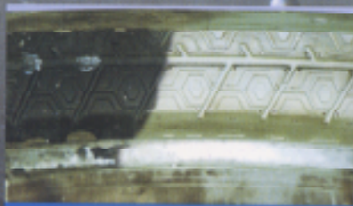
Rubber molders use CO 2 blasting to remove release agents and rubber residues from hot molds without removing them from the press.
